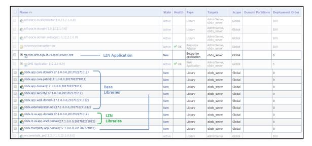
Figure 2: Deployments after OBDX 17.1.0.0.0 US LZN Installation
